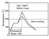
[Recommended condition for Pb-free soldering]
