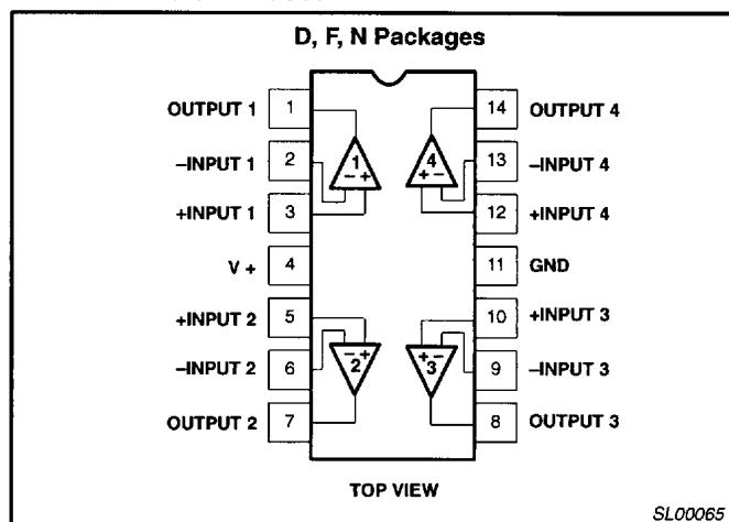
Figure 1. Pin Configuration
