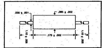
†Standard tolerance of 5, 10, and 20% are available — no suffix is ±20% tolerance, "A" suffix is ±10% tolerance, and "B" suffix is ±5.0% tolerance.
