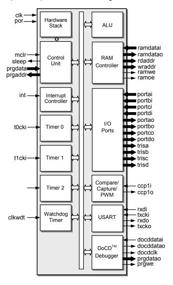
**Timer 0** – Main system's timer and prescaler. This timer operates in two modes: 8-bit timer or 8-bit counter. In the "timer mode", timer registers are incremented every 4 CLK periods. When the prescaler is assigned into the TIMER prescale ration can be divided by 2, 4 .. 256. In the "counter mode" the timer register is incremented every falling or rising edge of TOCKI pin, dependent on TOSE bit in OPTION register.
