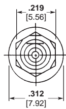
8-32 UNC-2A (Modified) Receptacle, Front Mount Part Number 145-0002-0001
