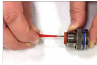
Plastic tool with contact in proper position.
