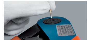
STEP 3: Insert the contact in the crimping tool.
