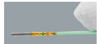
STEP 6: Inspect the contact. It must have 8 indents, and the wire must be seen in the contact inspection hole.
