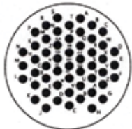
Series III Series II Series I No. of Contacts Service Ratings 23-53 22-53† 23-53 53 #20 I
