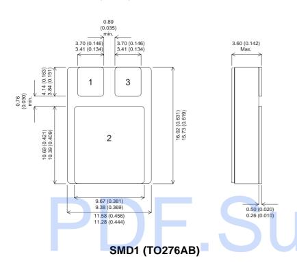
Bipolar NPN Device in a Hermetically sealed Ceramic Surface Mount Package for High Reliability Applications
