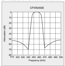
Note: To take best advantage of safety feature of ceramic filters, connect the output to an IF amplifier through a DC cut capacitor. Avoid directly applying a direct current to output of ceramic filters (between ⑤ and ②,③,④).
