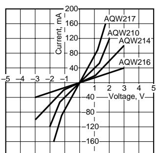
**9. Off state leakage current**
