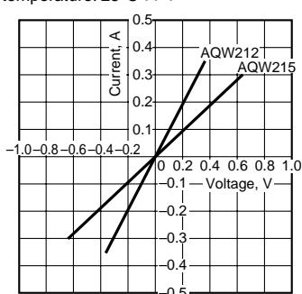
**8.-2) Voltage vs. current characteristics of output at MOS portion**
