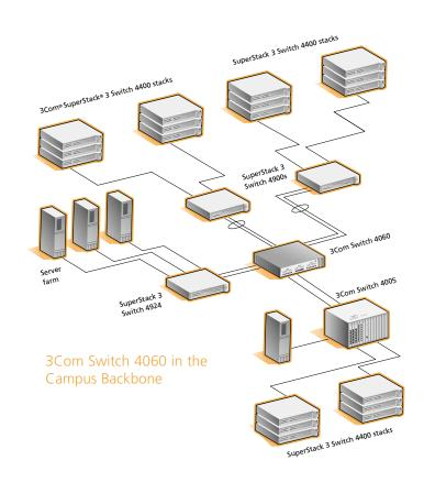
High-Performance Switching and Flexibility for the Backbone The 3Com Switch 4050 and Switch 4060, based on a 3Com-developed ASIC architecture, deliver 56 Gbps multilayer switching capacity for bandwidth-intensive core backbones and demanding enterprise applications. Each switch delivers non-blocking Layer 2 and Layer 3 switching across all ports, forwarding at speeds in excess of 40 Mpps.
