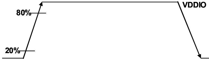
Figure 4. Output Pad Transition Waveform
