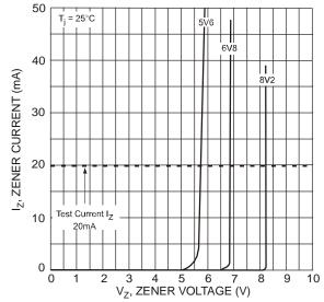
Fig. 2 Typical Zener Breakdown Characteristics
