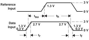
**VOLTAGE WAVEFORMS** SETUP AND HOLD AND INPUT RISE AND FALL TIMES
