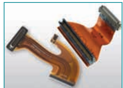
FLEX CIRCUITRY WITH RECTANGULAR CONNECTORS
