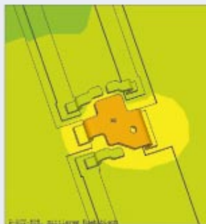
Lead frame of the SCT595-5-1 on a PCB with heat sink
