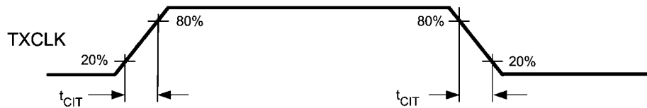
FIGURE 2. Transmit Clock Transition Times
