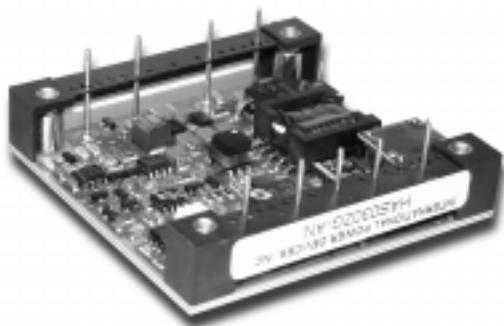
The HAS series is IPD's low cost industry standard half-brick converter. The HAS features a wide 2:1 input voltage, excellent efficiency, and IPD's open frame packaging technology. Operation is guaranteed from -40C to 100C, a built in input Pi filter insures low noise operation. Available in several input and output combinations, the HAS is perfect for industrial, telecom, and networking applications.
