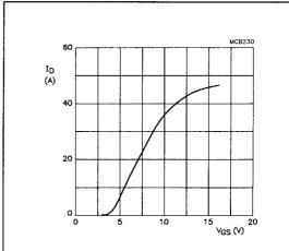
$V_{DS} = 10 \text{ V; } T_i = 25 \text{ }^{\circ}\text{C.}$
