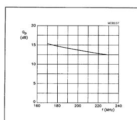
Class-A operation;  $V_{DS} = 28 \text{ V}$ ;  $I_{DQ} = 2 \text{ x } 4.6 \text{ A}$ ;  $R_{GS} = 82 \Omega$  (per section);  $T_h = 70 \, ^{\circ}$ C.
