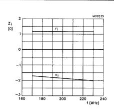
Class-A operation;  $V_{DS} = 28 \text{ V}$ ;  $I_{DQ} = 2 \text{ x 4.6 A}$ ;  $R_{GS} = 82 \Omega$  (per section);  $T_h = 70 \, ^{\circ}$ C.
