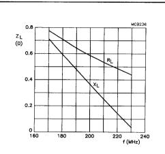
Class-A operation;  $V_{DS} = 28 \text{ V}$ ;  $I_{DQ} = 2 \times 4.6 \text{ A}$ ;  $R_{GS} = 82 \Omega$  (per section);  $T_h = 70 \, ^{\circ}C$ .
