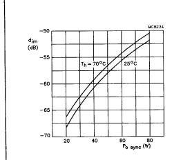
Fig.9 Intermodulation distortion as a function of peak synchronized output power.
