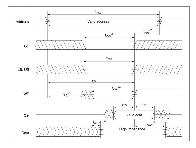
Write Cycle (2) ( $\overline{\text{CS}}$  Clock,  $\overline{\text{OE}} = V_{\text{IH}}$ )
