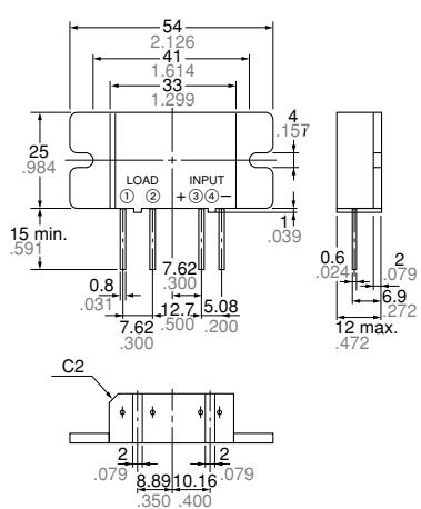
**Mounting hole location (Copper-side view)**
