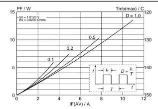
Fig.1. Maximum forward dissipation  $P_F = f(I_{F(AV)});$  square wave where  $I_{F(AV)} = I_{F(RMS)} \times \sqrt{D}$ .
