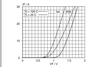
Fig.4. Typical and maximum forward characteristic  $I_F = f(V_F)$ ; parameter  $T_j$
