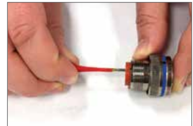
Plastic tool with contact in proper position.
