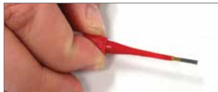
Plastic tool with contact in proper position.
