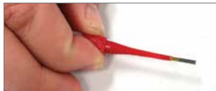
Plastic tool with contact in proper position.
