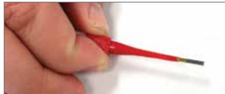
Plastic tool with contact in proper position.
