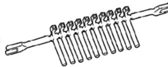
**Insulation Material:** Glass filled polyester. **Flammability:** UL94V-0. **Color:** Gray. **Contact Material:** Copper alloy. **Current Rating:** 1 A. **Insulation Resistance:** >5 x 10 Ω @ 250 VDC. **Temperature Rating:** -55°C to +85°C.
