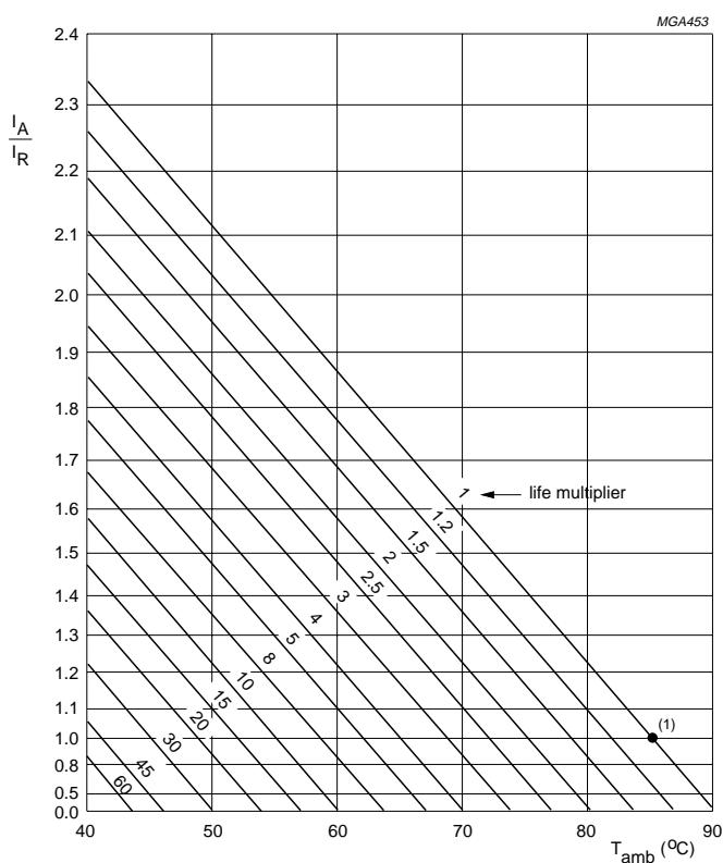
$I_A$  = actual ripple current at 100/120 Hz and 85 °C.
