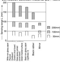
These bars indicate the sensing range with respective objects when the distance adjuster is set at the sensing range of 200mm,100mm and 50mm long, each, with white non-glossy
