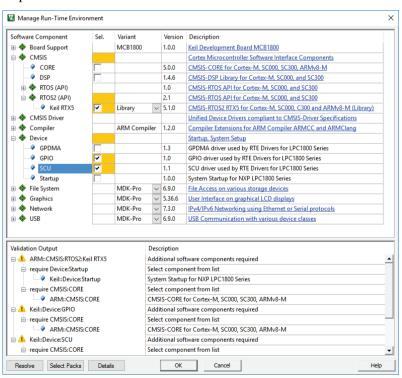
The Validation Output field shows dependencies to other software components. In this case, the components ARM::CMSIS:CORE and ::Device:Startup are required.
