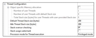
The Keil RTX5 kernel uses a separate stack space for each thread and provides two methods for defining the stack requirements:
