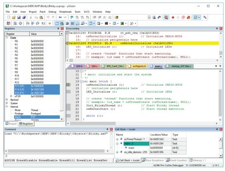
During the start of a debugging session,  $\mu$ Vision loads the application, executes the startup code, and stops at the main C function.
