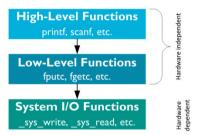
The high-level and low-level functions are not target-dependent and use the system I/O functions to interface with hardware.
