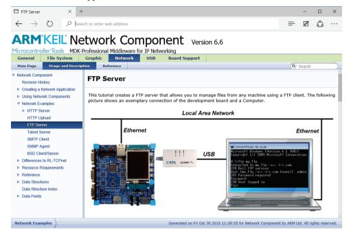
Several middleware components are the building blocks of this FTP server. A **File System** is required to handle the file manipulation. Various parts of the **Network** component build up the networking interface.
