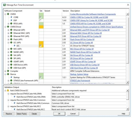
TIP: The links in the column *Description* provide access to the documentation of each software component.
