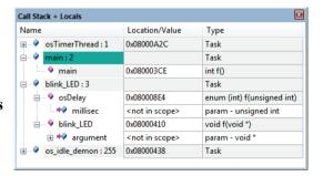
When program execution stops, the Call Stack + Locals window automatically shows the current function nesting along with local variables. Threads are shown for applications that use the CMSIS-RTOS RTX.
