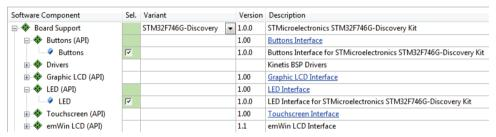
Be sure to select the correct **Variant** to enable the correct pin configurations for your particular development board.
