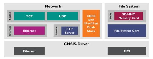
As explained before, CMSIS-Driver provides the interface between the microcontroller peripherals and the MDK Middleware.
