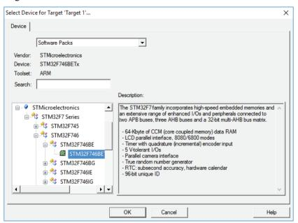
TIP: Only devices that are part of the installed software packs are shown. If you are missing a device, use the Pack Installer to add the related software pack. The search box helps you to narrow down the list of devices.
