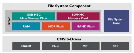
Each storage device is accessed and referenced as a **Drive**. The File System Component supports multiple drives of the same type. For example, you might have more than one memory card in your system.
