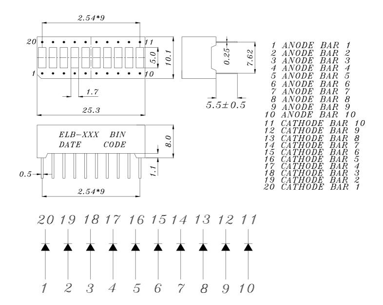
**Notes:** 1. All dimensions are in millimeters, tolerance is 0.25mm unless otherwise noted.
