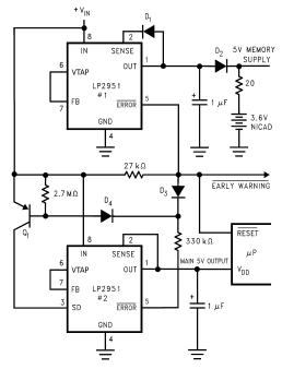
Figure 48. Regulator With Early Warning and Auxiliary Output
