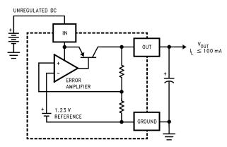
Figure 33. LP2950-N Functional Block Diagram
