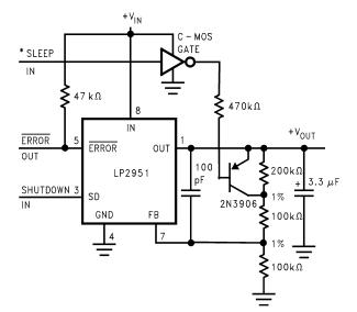
\*High input lowers V<sub>out</sub> to 2.5 V.
