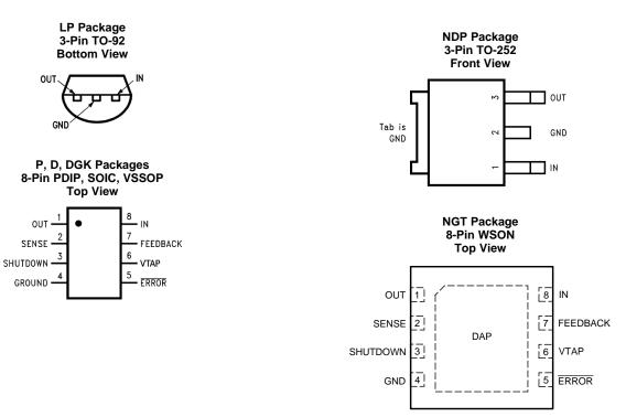
Connect DAP to GND at device pin 4.
