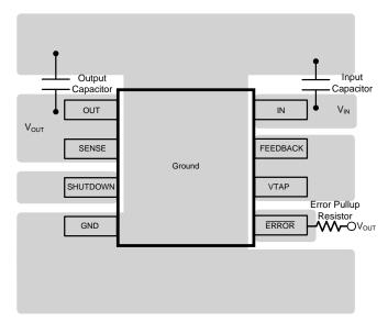
Figure 57. LP2951 VSSOP Board Layout
