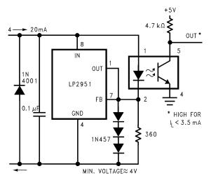
Figure 52. Open Circuit Detector for 4  $\rightarrow$  20-mA Current Loop
