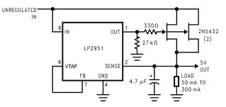
Figure 44. 300-mA Regulator with 0.75-V Dropout
