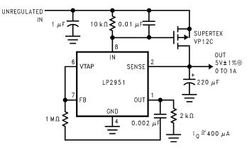
Figure 36. 1-A Regulator with 1.2-V Dropout
