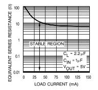
Figure 37. Output Capacitor ESR Range
