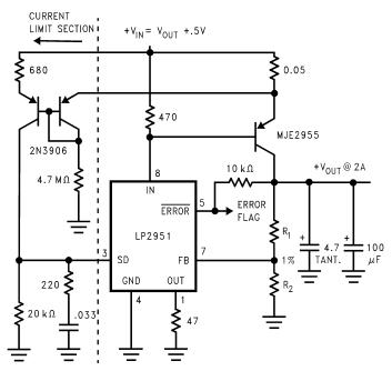
Figure 50. 2-A Low Dropout Regulator
