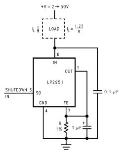
Figure 46. Low Drift Current Source
