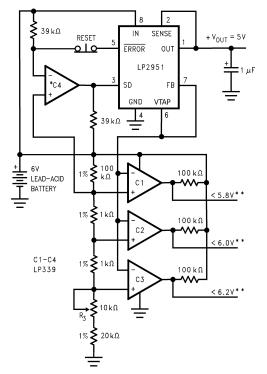
\*Optional latch off when drop out occurs. Adjust R3 for C2 Switching when V<sub>in</sub> is 6 V. \*\*Outputs go low when V<sub>IN</sub> drops below designated thresholds.
