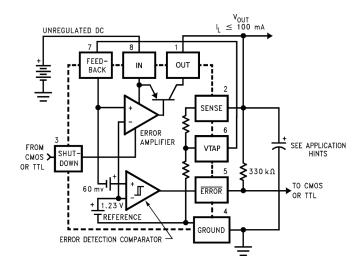
Figure 34. LP2951-N Functional Block Diagram
