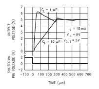
Figure 38. LP2951-N Enable Transient
