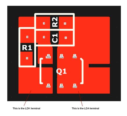
Each LASORB part formulation (i.e. the numbers which indicate the laser diodes that are best protected by LASORB) uses different values for R1, R2 and C1. *When ordering LASORB SMT KIT components, Pangolin has a minimum order quantity of 100 units per order. We also ask that you please discuss your laser diode protection requirements with Pangolin so that the most appropriate R1, R2 and C1 values are chosen and delivered to you along with Q1, the TSOP6/4G-20V semiconductor device.*
