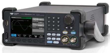
With 5 basic signal types, and over 40 built-in arbitrary waveforms the WaveStation is a versatile waveform generator. A variety of modulation schemes, intuitive waveform editing software and remote control capabilities, enable versatile waveform generation of waveforms up to 160 MHz. The large color display and simple user interface make it easy to generate a wide range of waveforms.
